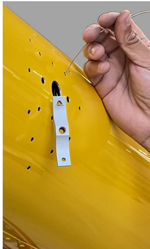
IMAGE 2 Installing F955-4 stiffener (RH side shown; LH side similar)
