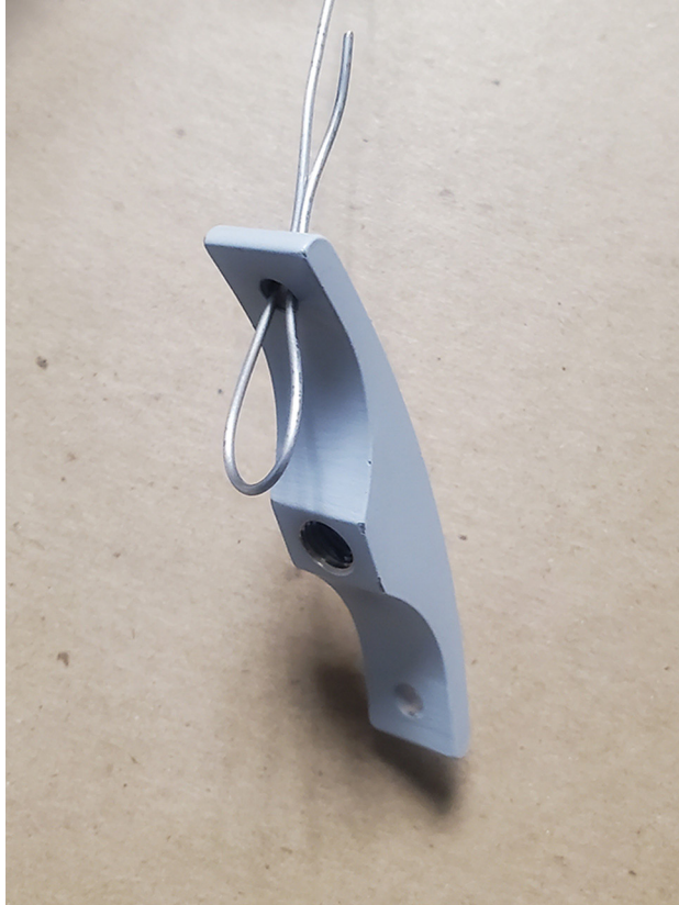
IMAGE 1 F955-4 stiffener & safety wire loop (shown with .040 inch thick safety wire)
