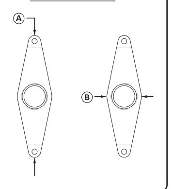
Using one-inch central conductor, rotate yoke at 120° intervals between inspections (3 inspections for this mode).
