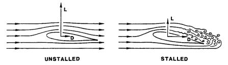
Wing or rotor blade unstalled and stalled.
