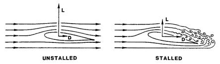
Wing or rotor blade unstalled and stalled.
