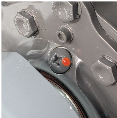
Reference Image: Factory-installed B569-1 Magnetic Plug
