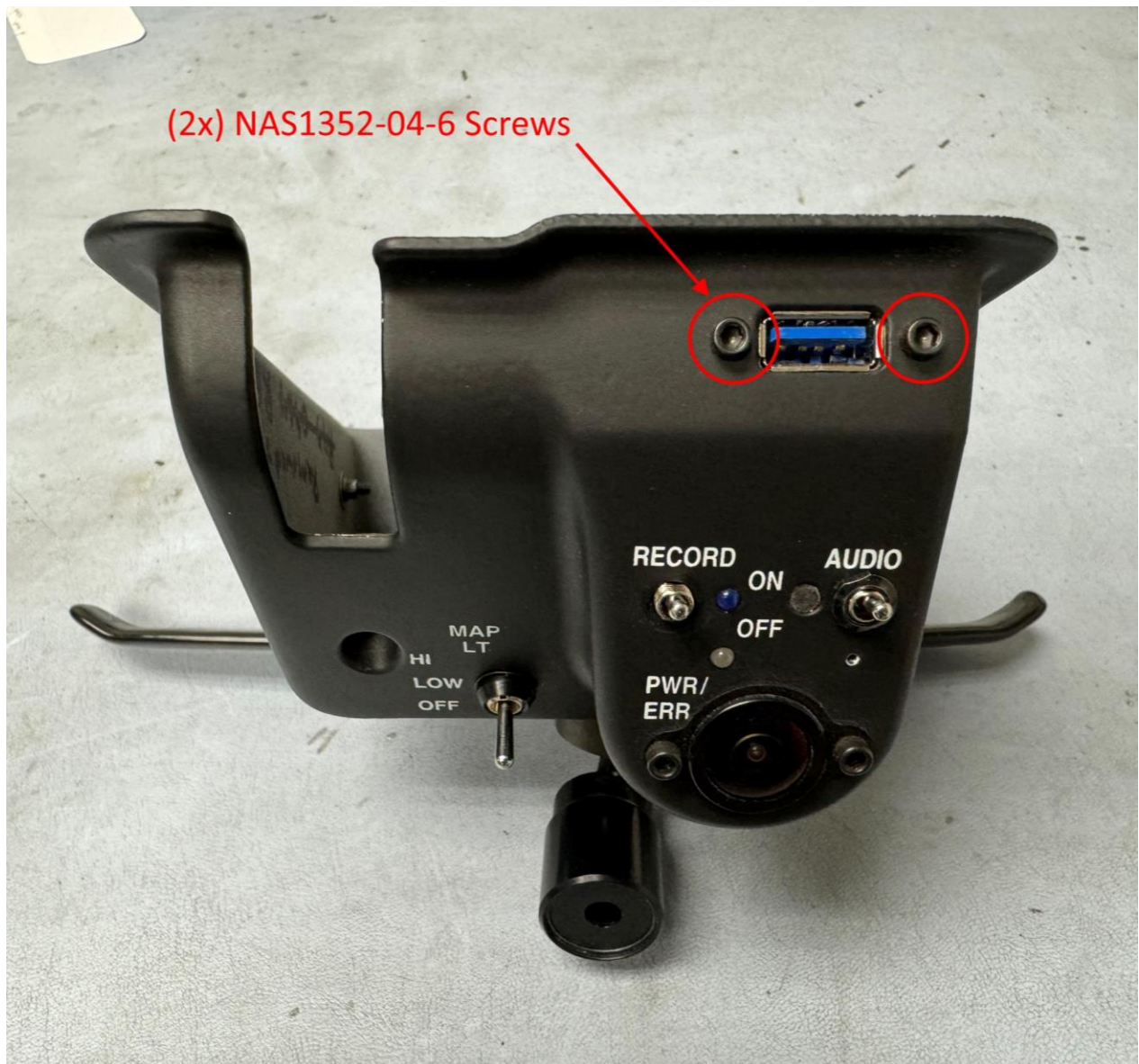
Figure 3: F039-2 USB Port Attachment Screws
