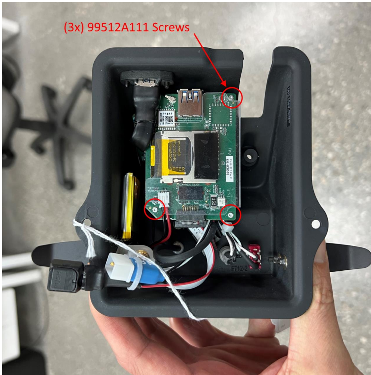
Figure 4: F039-2 Main Circuit Board Attachment Screws
